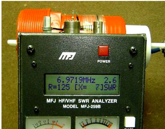
Fig1. Trap tuned to low resonance point
