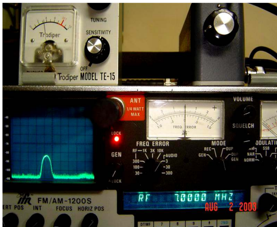
Fig3. GDO dip at 6.97MHz (50kHz/div)
