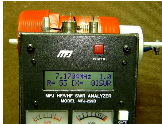
Fig2. Trap tuned to high resonance point
