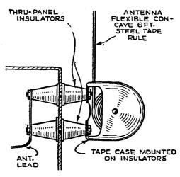
The familiar steel pocket rule of the concave type can be used as a variable length antenna as here shown.
