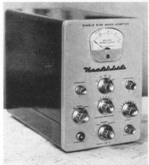
SB 10 SSB GENERATOR
