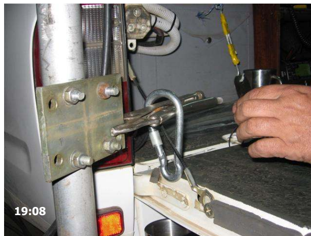
Improvised brake lock
