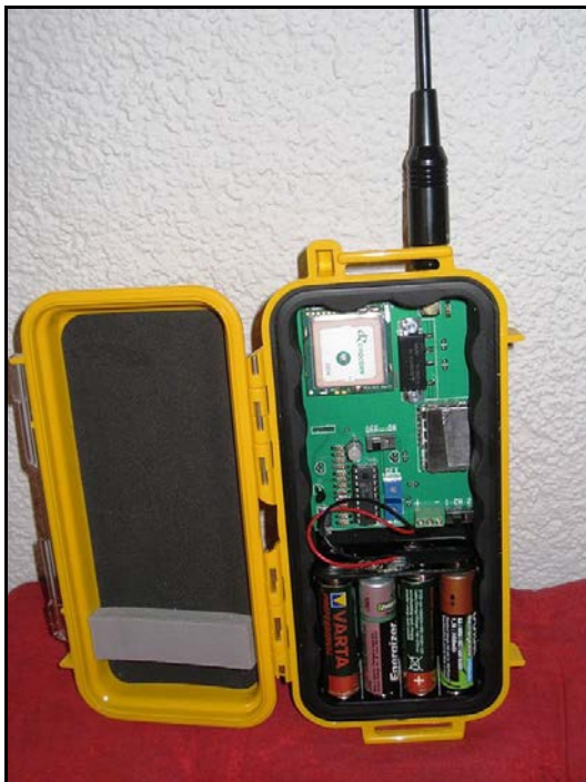
An APRS beacon transmitter with GPS receiver
