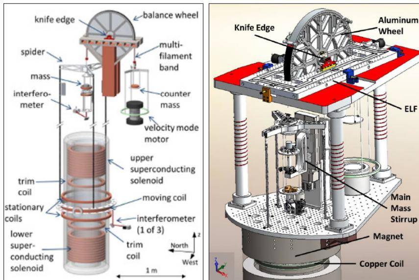
The Watt balance, or electronic kilogram, relates the kilogram to Planck's Constant. The NIST-4 (National Institute of Standards and Technology) consists of a copper wire coil suspended from one side of a precision made aluminium wheel balanced on a knife edge along the axle of the wheel. The hanging coil is immersed in a 0.55 Tesla magnetic field ( $\times 10\ 000$  greater than Earth's magnetic field), which is generated by a 1 ton SmCo permanent magnet.
